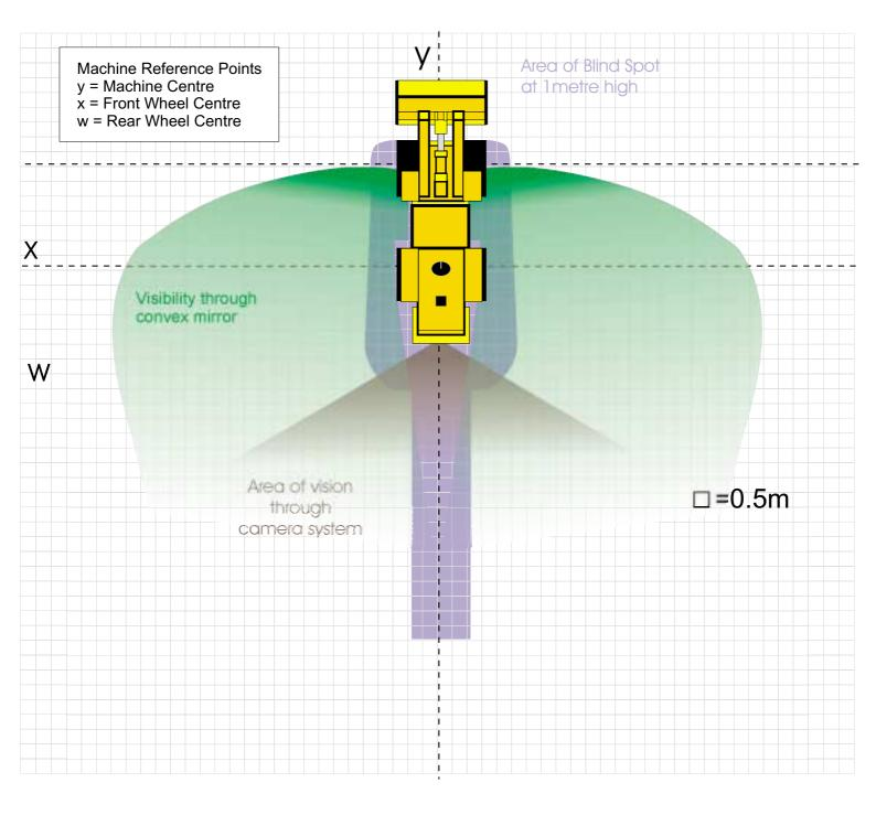
Recommendations 2 x NC100 Convex wing mirrors Arms will need extending or adjusting to see both flat and convex mirrors through obstructions
