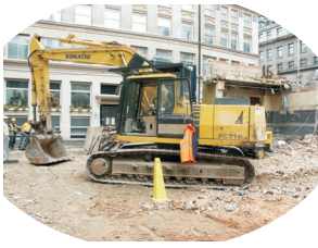
Komatsu PC210 Boom - Tracking Position
