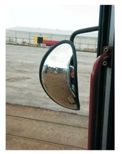
Off side, machine right I  $\times$  Nc I 00 - mounted on the existing mirror bracket to allow vision under the cab in a raised position
