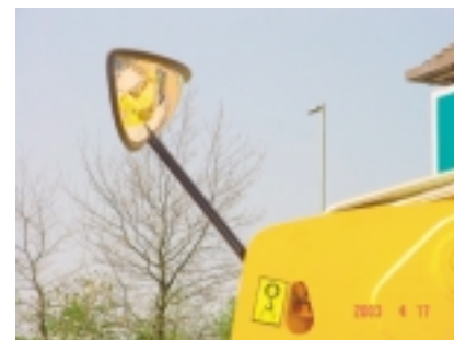
Convex mirror fitted to the rear of a telehandler (used in conjunction with a normal reversing mirror).
